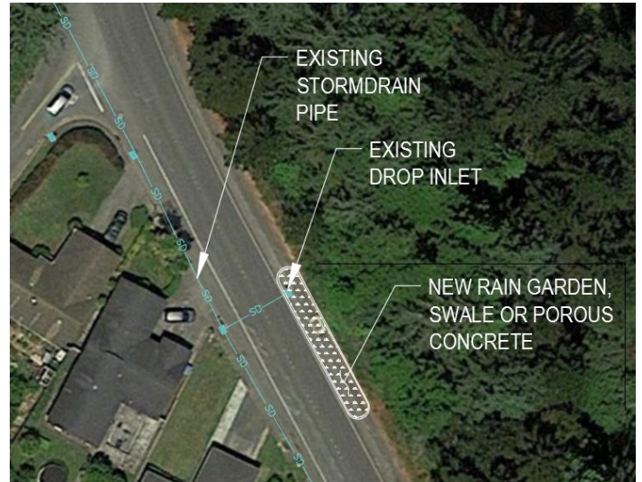
Image 2. Example Rain Garden/Bioswale at Roadway Shoulder
